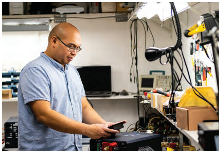
Francis Natividad, a technical specialist at Samlex, programs an EVO inverter/charger for a lithium battery using the Samlex EVO RC Plus remote control.
