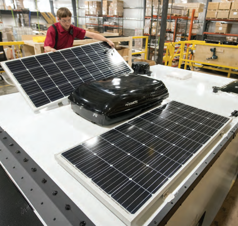
Ember Group Leader Verlin Hershberger installs a solar power panel on trailer. Solar power comes standard on Ember RVs, giving them the ability to go off-grid if its trailer owners desire.
