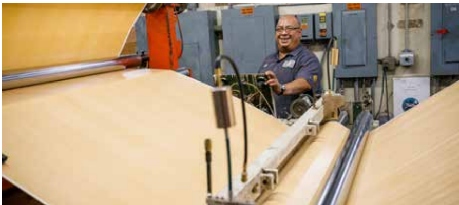
Robert Weed has five lamination machines that can laminate vinyl or paper overlay onto various substrates, typically plywood or MDF. Plywood laminated panels are used for interior walls of RVs. Laminated MDF is used in RV pocket doors and cabinetry.
