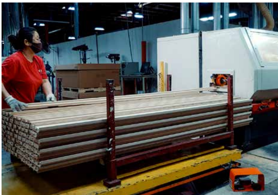
Robert Weed mills profiles for trim and molding pieces using a variety of saw machines. These trim pieces are used as door frames and other uses in RVs.
