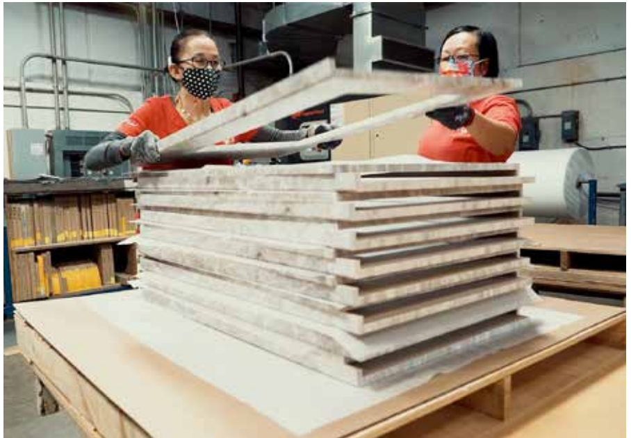
After the film overlay has been adhered to the substrate, the excess overlay is trimmed off and another quality control check is performed. This is part of the manufacturing process for RV countertops and sinks.
