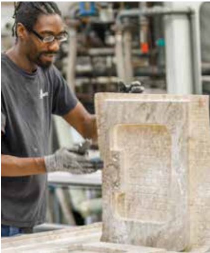
This is a sink manufactured using the rigid thermoform (RTF) process, which uses adhesive and vacuum pressure to secure the overlay to the substrate. This is often used to create countertops and sinks for RVs.
