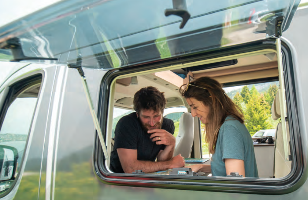
Polyplastic's acrylic windows have found favor in Europe because they weigh less than glass windows and they are very durable. (Photo courtesy of Lippert)
