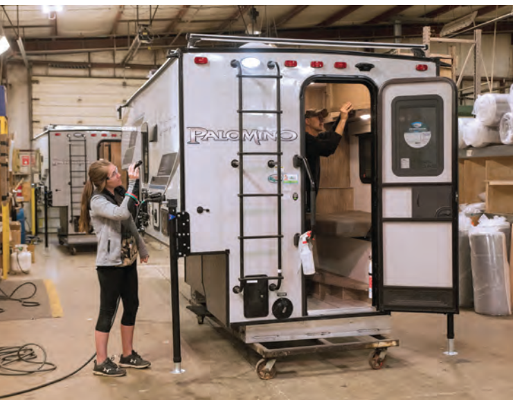
Team members Taylor Burbank and Dave Hostetler use flashlights to look for gaps, seal voids or imperfections during the inspection process.
