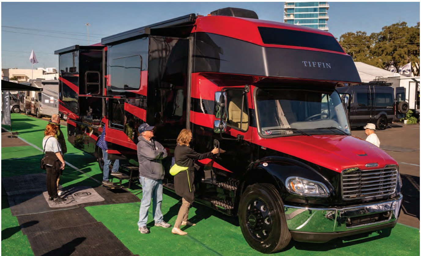
Tiffin's new Allegro Bay motorhome was a hit with attendees at the Tampa show. Freightliner created a customized S2RV chassis for the Allegro Bay, offering Tractech NoSPIN differential, which is designed to minimize or eliminate tire wheel spin in adverse conditions such as mud and snow.
