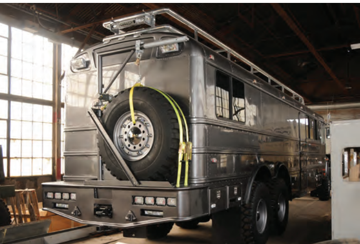
This converted bus, which has been highly modified inside and out, is called the Global Xplorer. A few highlighted product features include thermal imaging cameras, night vision surrounding the vehicle, custom specialized lighting, power spare tire retrieval and stow harness and central tire inflation system.
